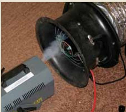
**Fog pinpoints leaks.** Forced into the ductwork by the duct blower, theatrical fog can track down both big and small leaks. It's also a good way to silence HVAC installers convinced that their ducts are sufficiently sealed.
